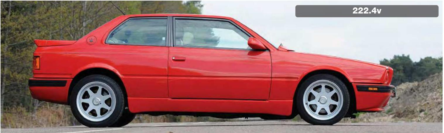
The standard Biturbo package was potent, but it's not the Italian way to settle for merely potent; faster is always better. The early go-faster Biturbo was the 'S', which first introduced intercooling to the model – and nifty NACA ducts to the bonnet. Designed for the Italian market, it packed 205hp compared to the standard car's 185hp, and featured stiffer suspension, two-tone bodywork and wider tyres.
